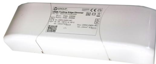
The CASA trailing edge dimmer is a trailing edge dimmer. Its use enables stepless dimming of trailing-edge lamps. Output power 150W LED / 200W ohmic (e.g. light bulbs). It is controlled wirelessly with the CASAMBI® app. Strain relief and terminal cover are integrated.
